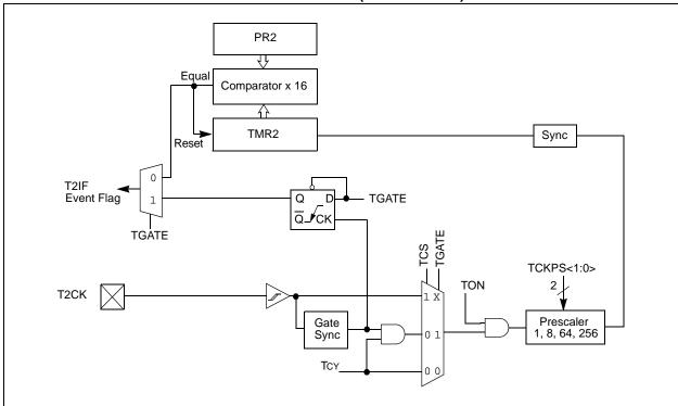
FIGURE 11-3: 16-BIT TIMER3 BLOCK DIAGRAM (TYPE C TIMER)
