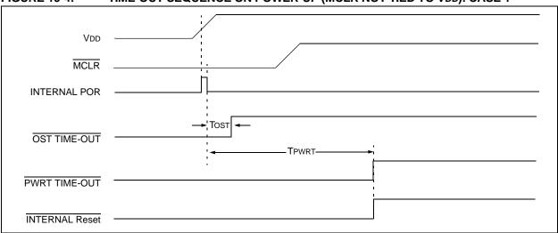
FIGURE 19-5: TIME-OUT SEQUENCE ON POWER-UP (MCLR NOT TIED TO VDD): CASE 2
