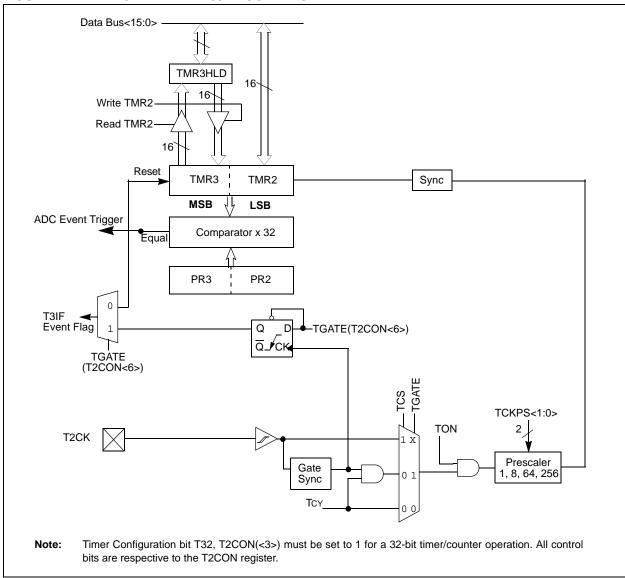
FIGURE 11-2: 16-BIT TIMER2 BLOCK DIAGRAM (TYPE B TIMER)
