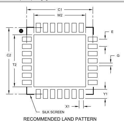
**MILLIMETERS** Units **Dimension Limits** MIN NOM MAX Contact Pitch 0.65 BSC Ε Optional Center Pad Width 4.70 W2 T2 4.70 Optional Center Pad Length 6.00 Contact Pad Spacing C1 Contact Pad Spacing C2 6.00 Contact Pad Width (X28) X1 0.40 Contact Pad Length (X28) Υ1 0.85 Distance Between Pads G 0.25
